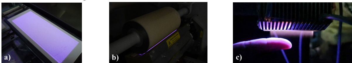
Fig. 1. Photographs of discharges used for the plasma treatment of fabrics for FRP composites: DCSBD (a) and VDBD (b) generated in ambient air, and a DCSBD linear APPJ (c) operating with N 2 into ambient air.
